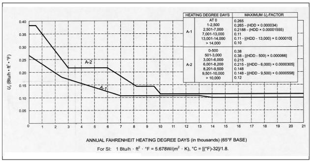
• Figure 3 Uo – Overall U-factor Compliance Lines, by Heating Degree Days (A-1 = One and Two-family Dwellings, A-2 = Other Low-rise Residential Buildings) Calculating Wall Thermal Values
